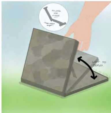
Product is deployed by lifting the top tile layer until locks at 75-degree angle.
